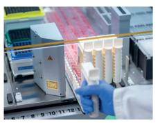
Fast and simple sample loading and identification with Fluent ID
