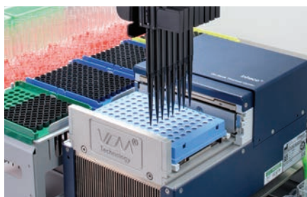
Pipetting directly into thermocycler*
