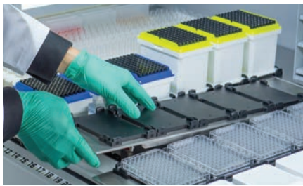
Exchange deck segments for flexible assay set-up, device integration and reconfiguration
