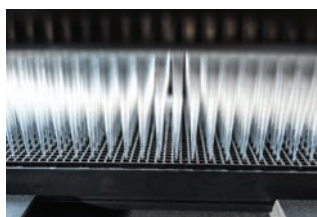
MCA 384 with disposable tips pipetting to 1,536-well microplate
