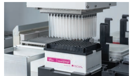
Multiple Channel Arm picking up 96 500 \mu\text{l} disposable tips
