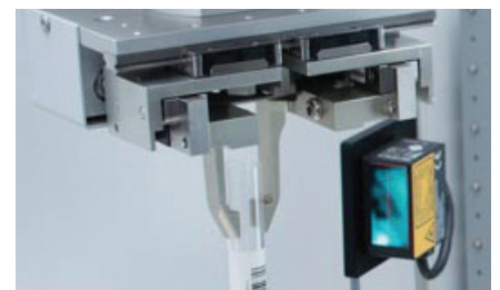
Tube handling with Robotic Gripper Arm
