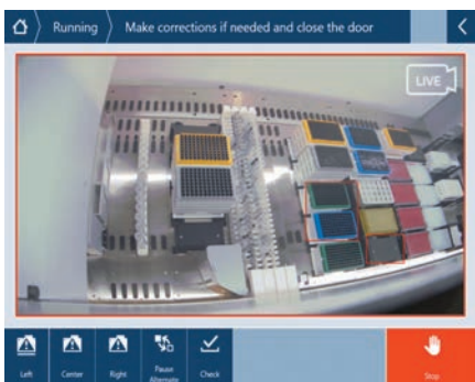
DeckCheck highlights differences to the expected worktable
