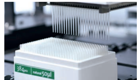
Multiple Channel Arm picking up one row of 24 50 \mu\text{l} tips
