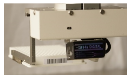
Plate handling with barcode reading
