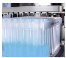
8-channel, dual pump dispense head provides high throughput and reduces processing times
