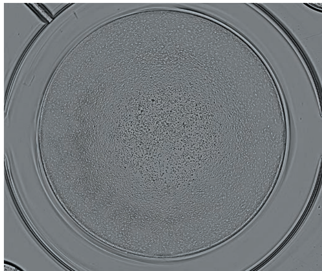
Single image of an entire well from a 96-well plate. No tiling or edge-to-edge optical distortion leads to superior results when analyzing cell populations.
