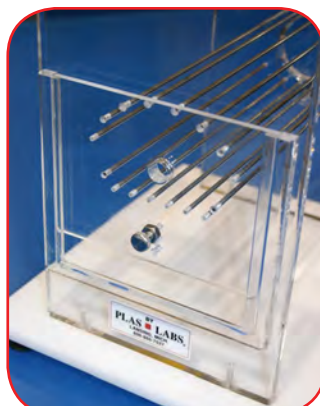
Door in the upper position locks the stainless rods in place.
